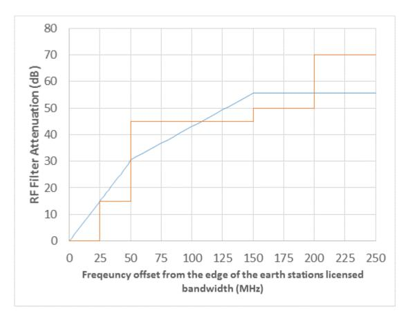
Orange line - RAG Tx 3.4 GHz Table 1 Blue line - Corrected Table 1, aligning with FCC mask
