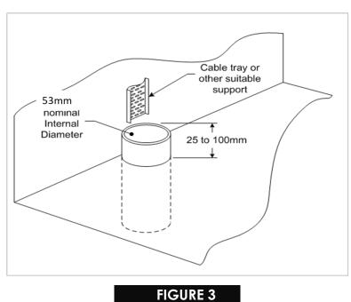
Sleeve example telecommunications riser/closet floor or ceiling entry
