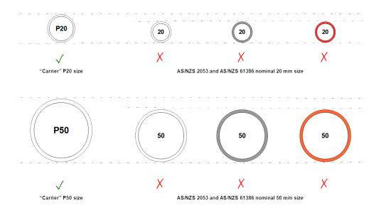
Note: The conduit sizes defined in this Guideline derive from AS/NZS 1477. These sizes are used by telecommunications carriers. Refer to the Definitions section for dimensions of these P20, P50 and P100 "carrier" conduits.
