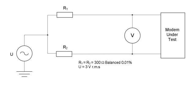
Figure 3 Impedance balance test circuit
