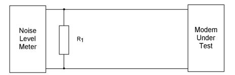
Termination provided by Noise Level Meter, or external resistor R1= 600  $\Omega\,\pm\,1\%$
