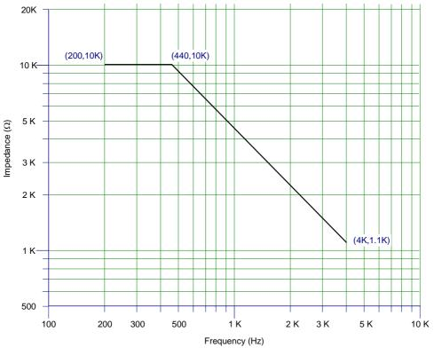
Note: Between 440 Hz and 4 KHz the log of the impedance decreases linearly with the log of the frequency.
